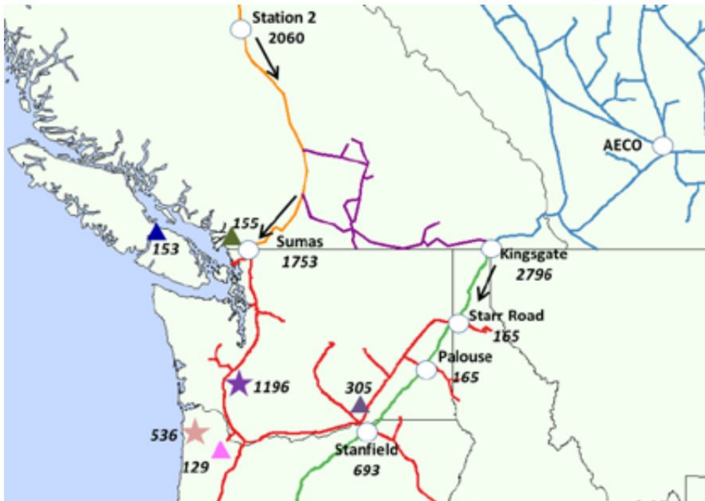
Figure C1. Northwest Infrastructure and Capacities (MDth)
